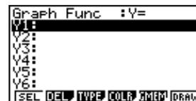
Many of the operations performed by this calculator can be executed by pressing function keys **[F1]** through **[F6]**. The operation assigned to each function key changes according to the mode. Function menus are at the bottom of the display in each mode.
